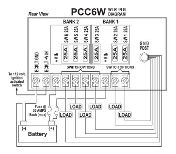
**BCKLT +V:** This terminal supplies power to the units window backlighting. This terminal can be connected to any ignition controlled +VBAT power source that can supply 100ma.
