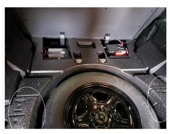
STEP 2: REMOVE THE FLOOR SURROUND SECTION AS SHOWN WHICH WILL EXPOSE THE CROSS BRACE UNDERNEATH IT.
