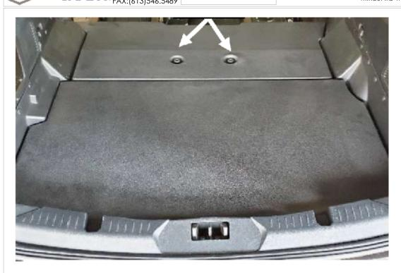
STEP 1: REMOVE BOTH THE SECTIONS OF OEM TRUNK FLOOR BY REMOVING THE BOLTS AS SHOWN.
