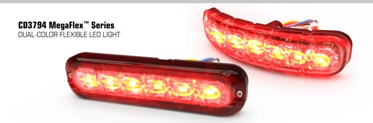
Code 3's MegaFlex™ is a versatile exterior warning light that can be mounted on flat or curved surfaces up to 120° with self-adhesive, very high bond tape. Its 12 dual-color LEDs provide exceptional output with combinations of amber, white, blue and red colors available. The light heads are protected in a clear, silicone housing that can flex while resisting yellowing and warping. A two-bolt bezel is also included for easy installation on flat surfaces.
