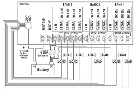
**BCKLT +V:** This terminal supplies power to the units window backlighting. This terminal can be connected to any ignition controlled +VBAT power source that can supply 100ma.
