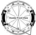
Remove 4 screws and remove brackets
