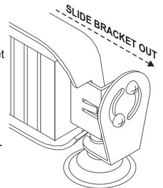
**NOTE:** If you replace the lens on the side of the power cord, make sure the cord is in its wire channel before re-attaching the suction cup assembly.
