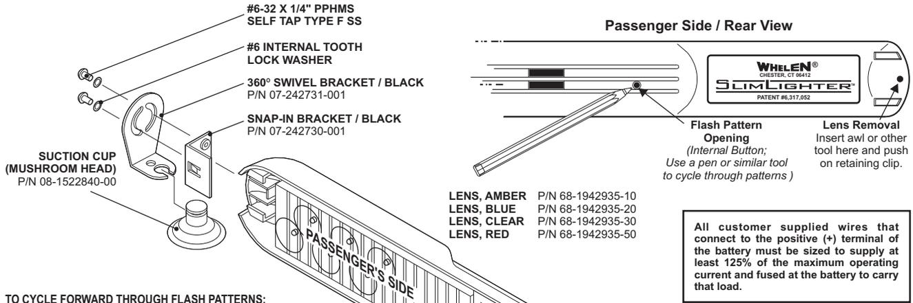
All customer supplied wires that connect to the positive (+) terminal of the battery must be sized to supply at least 125% of the maximum operating current and fused at the battery to carry that load.
