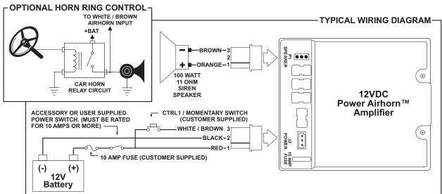
**WARNING:** All customer supplied wires, that connect to the positive terminal of the battery, must be sized to provide at least 125% of the maximum operating current, and fused "at the battery" to carry that load.
