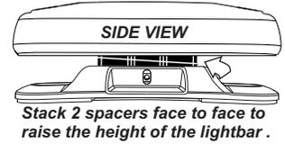
**Lightbar angle:** Place the lightbar onto the vehicle roof in its exact mounting location and use a level to check the angle of the lightbar. If (because of the curvature of the vehicle roof) the front and rear lights project up or down, you will need to install one of the supplied spacers. Note the angle of the tilt to determine where to place the spacer. **Installation:** Remove the mounting feet and install the spacer (maximum 1 per side) then reinstall the feet.
