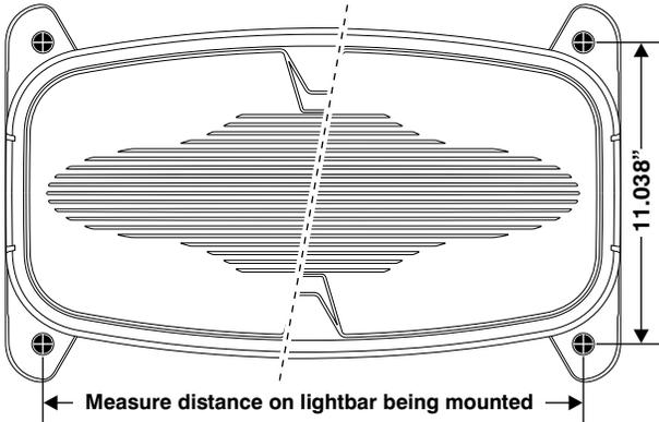
1. Install the mounting foot to the lightbar following steps 1 thru 4 of "Strap Mounting".
