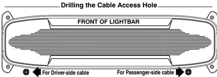
1. To protect the headliner from damage caused by drilling the cable access hole through the vehicle roof, allow a 5" to 7" distance between roof and headliner by lowering the headliner before drilling.
