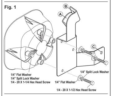
IMPORTANT: For drainage purposes, the speaker must be oriented so that the wire passage hole is in the "6 o'clock" position (closest to the road). This is also the drain hole for the siren. Improper mounting will result in premature driver failure and void the product warranty.
