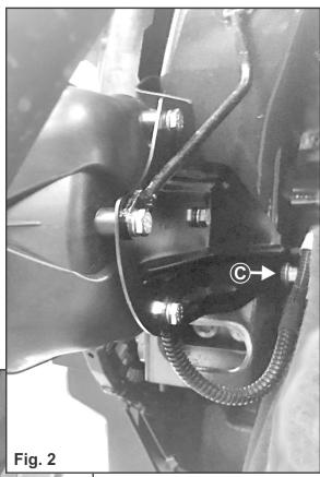
3. Using Existing Hardware: Mount the bracket with speaker to the vehicle. To locate the mounting holes you will use, refer to figures 2 and 3 for the location of the existing holes to mount to. Figure 1 shows the tabs on the bracket that correspond to the mounting holes.
