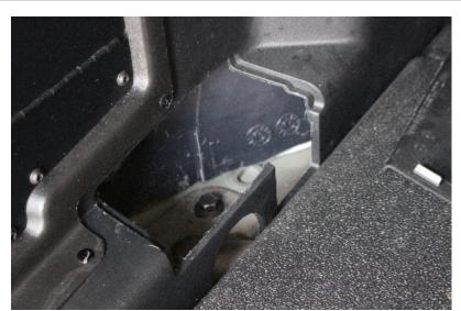
STEP 1: REMOVE PLASTIC COVERS FROM FORD INTERCEPTOR CROSS-BRACING (BOTH SIDES) AND REMOVE THE FORWARD MOST BOLT FROM CROSS-BRACE (BOTH SIDES) WITH 15mm SOCKET.
