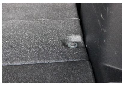
STEP 2: REMOVE THE BOLTS SECURING THE CARGO FLOOR (BOTH SIDES) USING 10mm SOCKET
